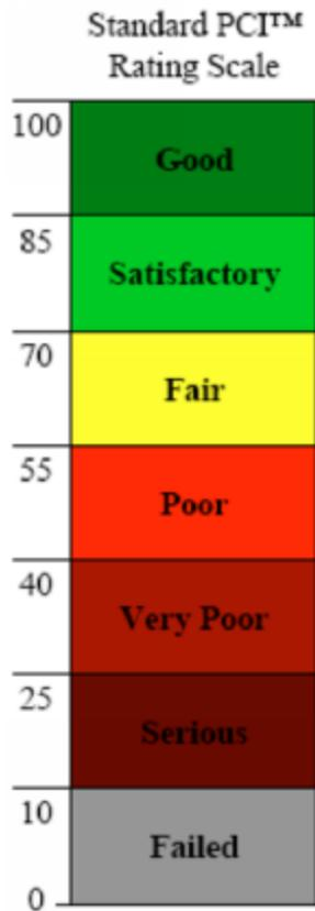
**Figure 1—Pavement Condition Index Values**
